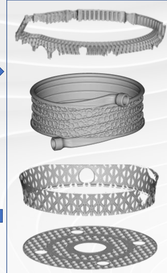
Lattice, surface texture and automated design tools (Designed in nTopology)
